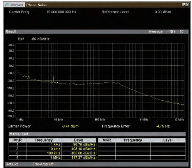
Phase Noise Measurement 79 GHz Measurement Frequency (Using High-Performance Waveguide Mixer MA2808A)
