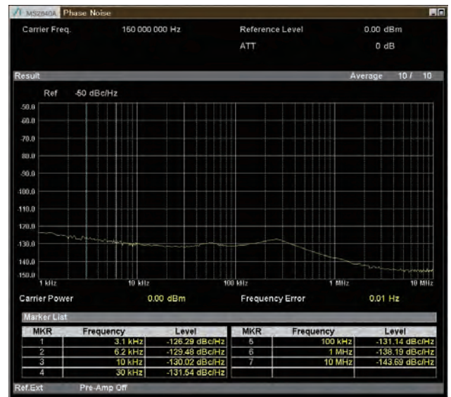
Phase Noise Measurement 150 MHz Measurement Frequency, Preamp Off
