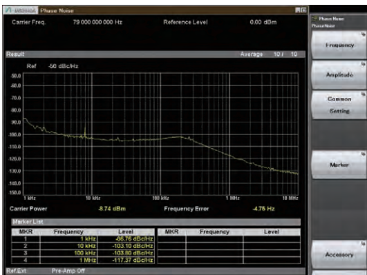
Phase Noise Measurement 79 GHz Measurement Frequency (using High Performance Waveguide Mixer MA2808A)
